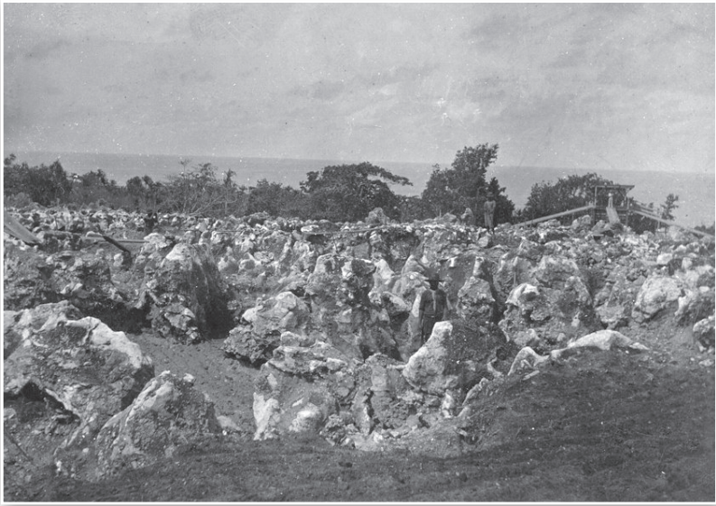
Extraction of rock phosphate, a product of bird droppings, left a field of pinnacles when the deposit was worked out.
